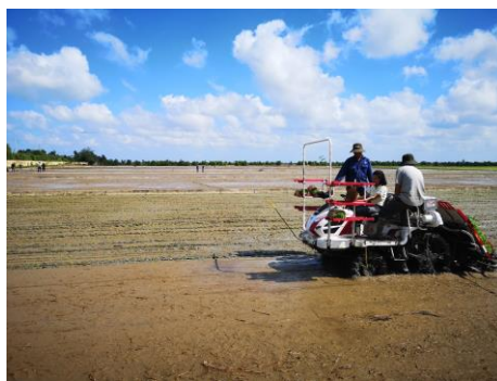
Figure 28. Transplanting rice by use of mechanical transplanter
