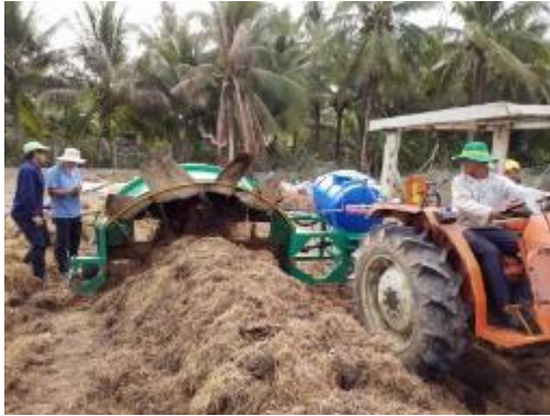
Figure 36a. Compost turner—front view.
