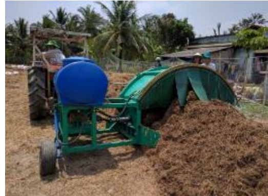
Figure 36b. Compost turner—rear view.
