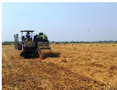
Figure 26. Self-propelled round baler (left) and loose straw collecting machine (right).
