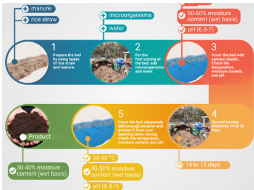
Figure 30. Step-by-step mechanized rice straw composting
