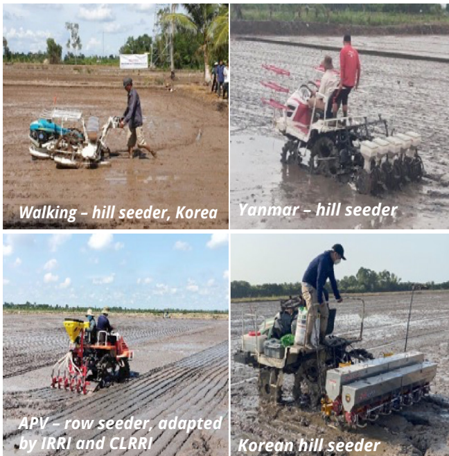
Figure 13. Typical wet-mDSR machines being tested in MRD
